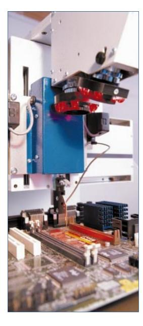
If you need to work on a board with a power distribution fault, the GRS will help you safely identify these types of fault before you apply power .
