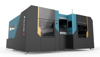
Falcon X is the flag ship model of the Falcon series. It provide extreme production capacity. A very unique design with double system machine equipped with a special loading mechansim in middle allows it to load inner layers to the left and the right side system. This innovative design allows the machine to process two separate stacks of PCB at the same time.
