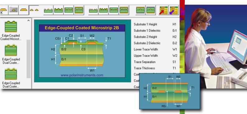
Boundary element method field solver includes modeling for multiple changing parameters and local resin rich areas
