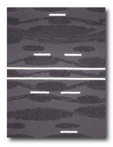
waveguide is designed with very close spacings, almost all of the electric field occurs in the horizontal gap between the traces. Defining local variations in E<sub>r</sub>, therefore, is crucial for the highest accuracy in predicting impedance.
