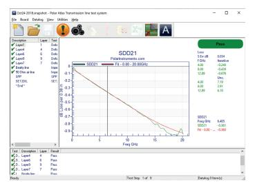
Atlas Si is a precision insertion loss measurement package designed specifically for PCB fabricators and OEMs. It provides accurate, repeatable measurements of frequency based transmission line losses, allowing fabricators to meet stringent targets that maintain signal integrity within the limits of the latest high-speed chipsets.
