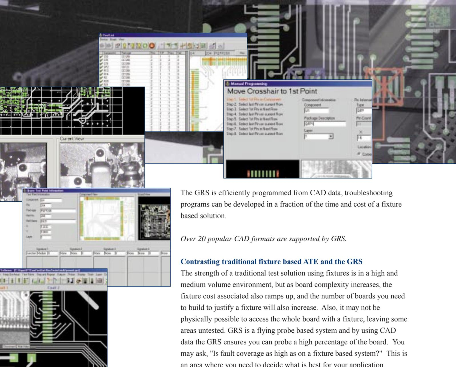
The GRS is efficiently programmed from CAD data, troubleshooting programs can be developed in a fraction of the time and cost of a fixture based solution.
