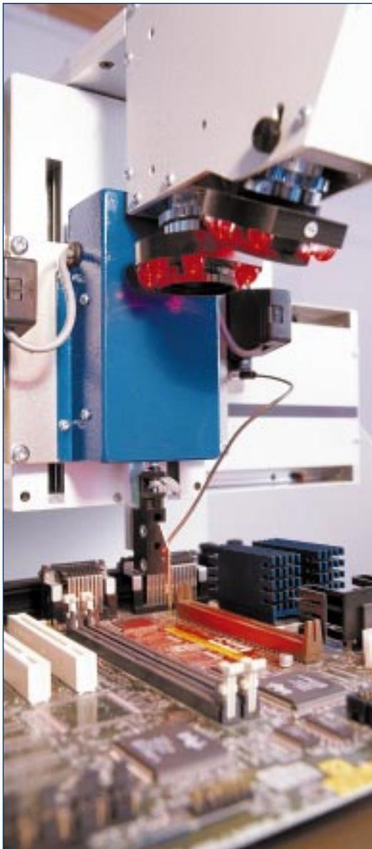
If you need to work on a board with a power distribution fault, the GRS will help you safely identify these types of fault before you apply power .
