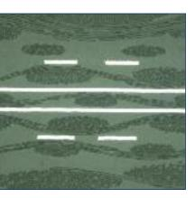
This photograph illustrates a polished microsection of a typical glass resin composite structure. This is FR4 but could equally be any woven glass reinforced composite. Glass has a dielectric constant of 6, the resin around 3. With high frequency base materials the resin Er can be even lower. On fine geometry boards with differential traces, local variations in the material Er need to be taken into account to obtain the most accurate prediction of impedance.
