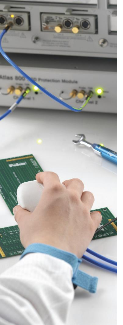
Atlas is compatible with commonly specified test techniques for TDR-based insertion loss (SDD21) measurement, Delta-L, SET2DIL & SPP.
