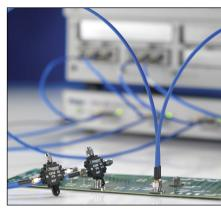
Atlas includes SET2DIL testing of frequency-based insertion losses – SDD21 and S21
